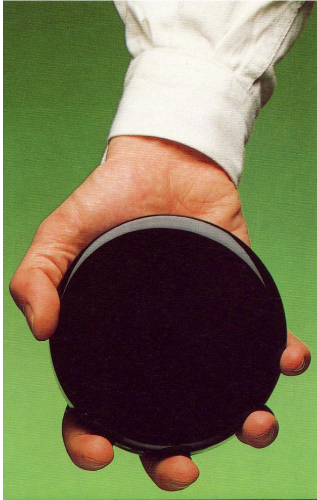
This glass disc simulates the amount of vitrified waste produced by one person in a lifetime if all his electricity was produced by nuclear energy.
